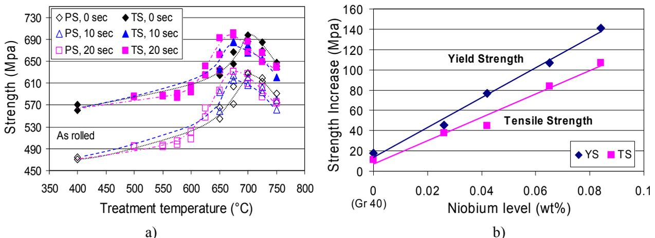
Fig. 3 a) Laboratory age hardening of 0.084% Nb UCS steel and b) Strength increase between the hot rolled and maximum age hardened strengths as a function of Nb level [3]
