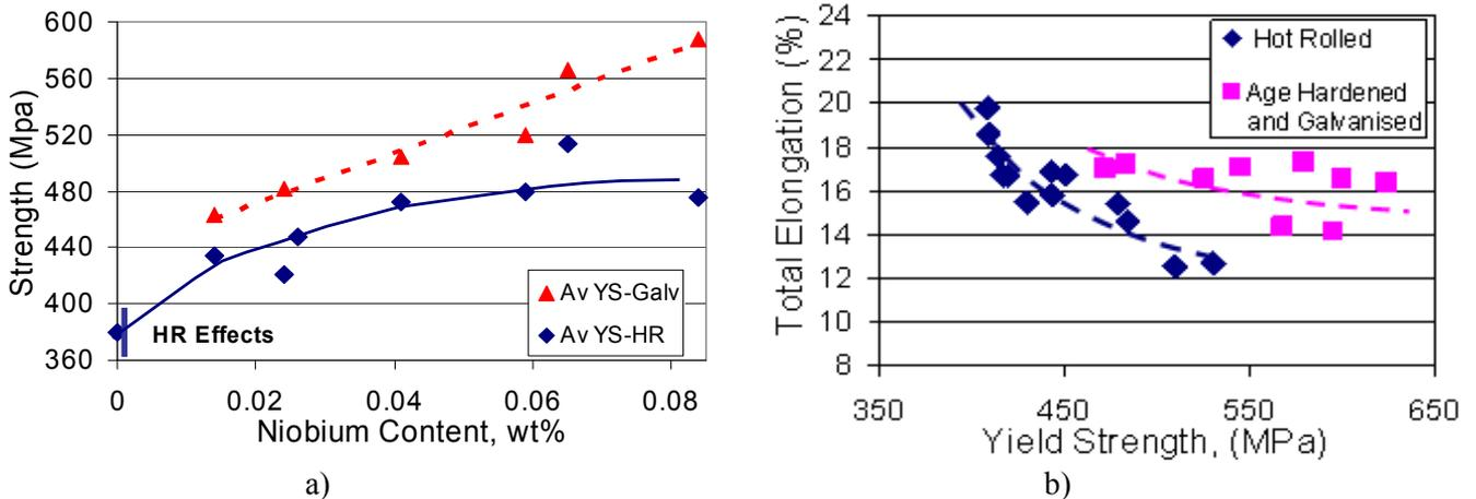
Fig. 4 a) Age hardening response of Nb UCS steels as a function of Nb content, b) Comparison of total elongation results between hot rolled and age hardened and galvanised Nb microalloyed UCS steels
