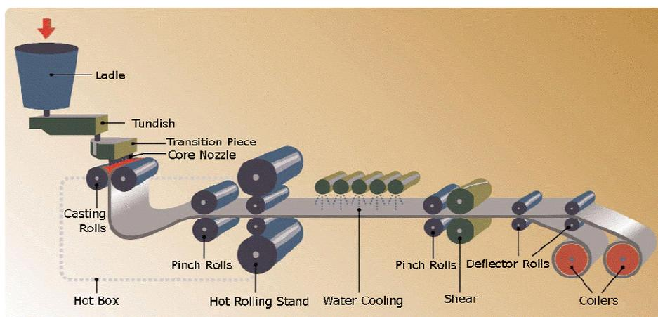
Fig. 1 Main components of the CASTRIP® process
