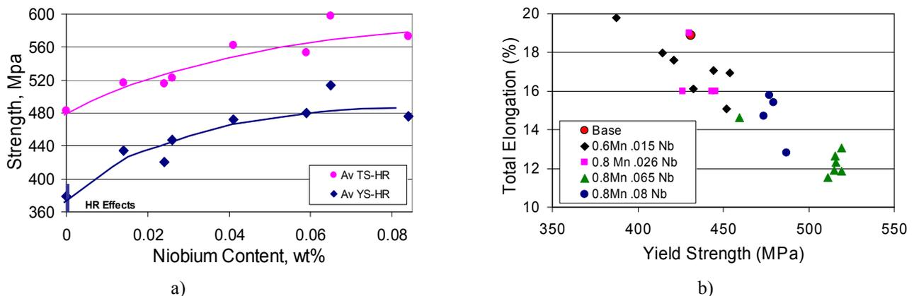
Fig. 2 a) Effect of niobium content on the average yield and tensile strength of hot-rolled Nb UCS steels. b) The change in total elongation with yield strength for Nb UCS steels
